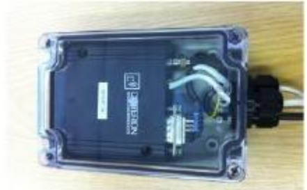
Remote GSM modem – Dust monitor end.
