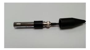
1. Connect the BNC plug from one end of the double booted cable to the microphone's BNC socket.
