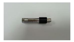
Make sure the ACO 7146 Class 1 microphone has the rubber sleeve fitted as shown in the above photograph. If it isn't the rubber boot will not provide a waterproof connection. The Turnkey Class 2 microphone does not require the sleeve but has a machined step instead.
