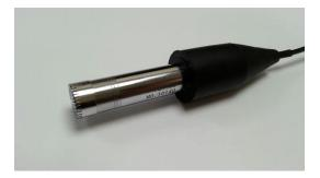
2. Next, ease the flexible rubber boot over the connector and rubber sleeve.
