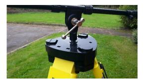
2. Screw the Microphone Clip to end of Boom.
